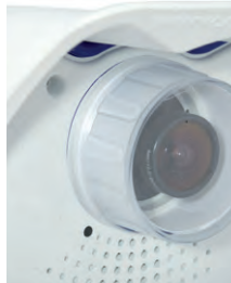
The white ring in the lens cover prevents the camera LEDs from adding light reflections to images
