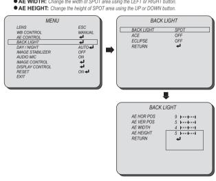
Select BACK LIGHT using the UP or DOWN button and enter using SEL button.
