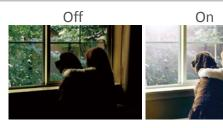
foreground. No matter if the main object is moving toward left, right, upper, lower, or any location in the screen, BLC provides perfect exposure for an object in front of strong back light
