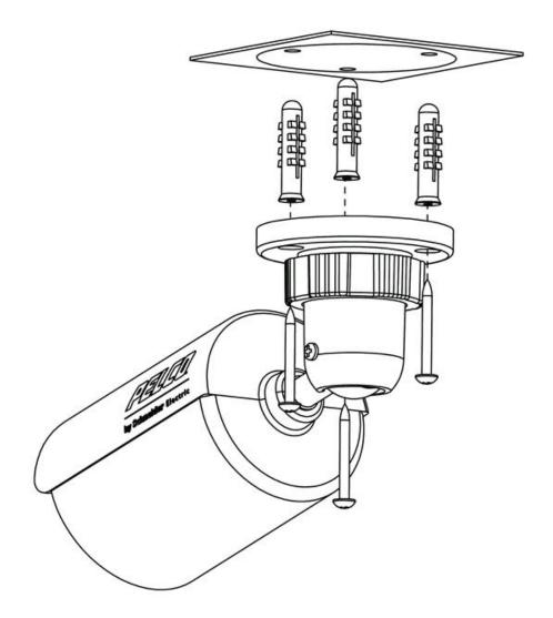
**Figure 2-1 Mounting the Bracket**
