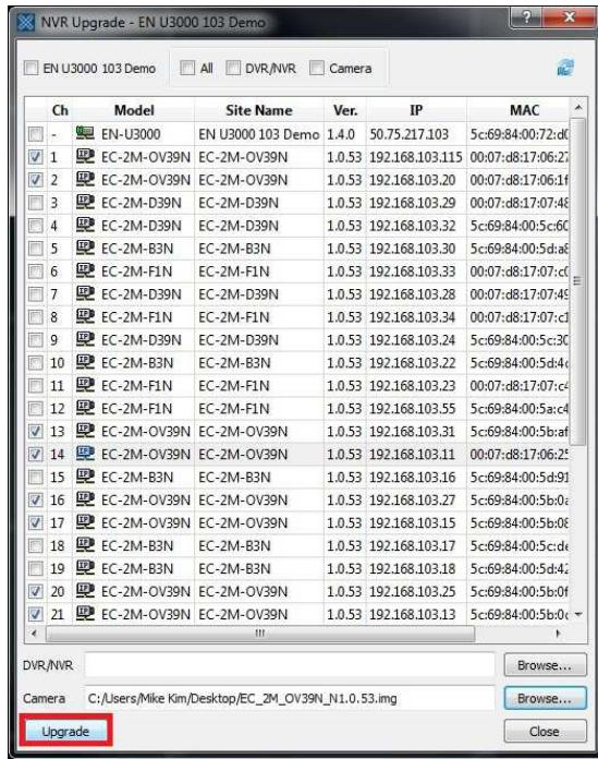
8. Upgrade will upload the firmware into the cameras from the upgrade and will begin its upgrade process in chronological order from the list.
