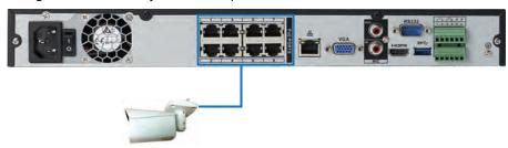
Connect IP cameras directly to PoE ports.
