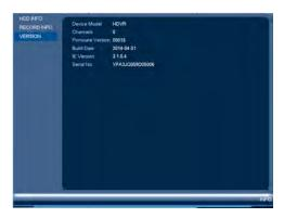
The Version sub-menu allows you to view information about the current firmware installed on the system.
