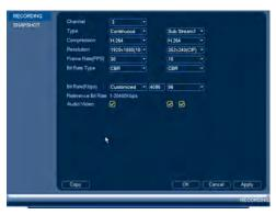
Resolution: Select the resolution that you want to use to record the selected channel. Higher resolutions create a more detailed image, but take up more hard drive space to record and require more bandwidth to stream to connected computers or mobile devices.
