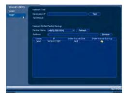
The Test menu allows you to test if your system can connect to other devices over the LAN or Internet. You can enter the IP address of a device and click **Test** to determine if your system can connect to it.
