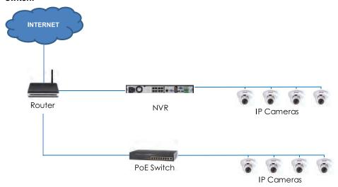
Connect an Ethernet cable from the LAN port on an external PoE switch (sold separately on <a href="www.flirsecurity.com/pro">www.flirsecurity.com/pro</a>) to your router using a CAT5e or higher Ethernet cable. Connect the power cable to the PoE swtich and to a power outlet or surge protector.
