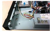
5. Turn the system over carefully. Tighten the hard drive screws (4x) to secure the hard drive.
