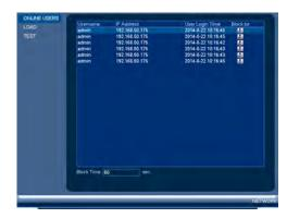
The Online Users menu shows a list of users connected to the system using computers or mobile devices.
