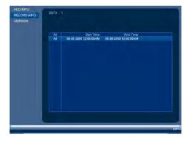
The Record Info menu shows the start and end times of recordings saved on the hard drive.
