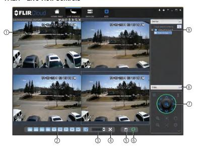
Live display: Double-click to expand the area. Right-click to access additional options. Hold the mouse over the display area to access the camera toolbar.
