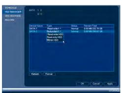
2. Click the **Type** drop-down under the second hard drive and select **Mirror HDD**.
