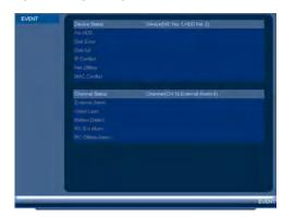
The Event Info menu shows you a display of system alarms. Activated alarms are highlighted in white. Additional info such as channels that are currently detecting motion is shown.
