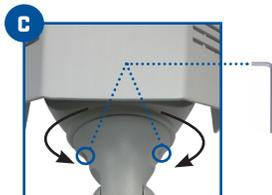
C) Loosen the screws on either side of the camera stand with the Allen key to rotate the camera housing. Loosen the right-side to make fine adjustments, or the left-side for broad adjustments.
