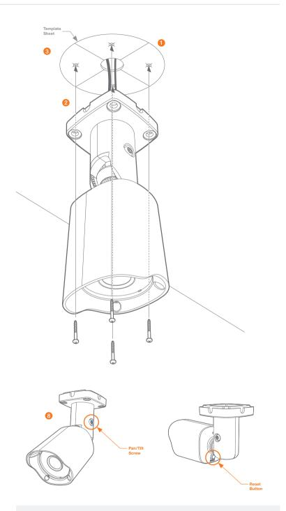
Resetting the camera: To reset the camera, use the tip of a paper clip or a pencil and press the reset button. Pressing the button for five (5) seconds will initiate a camera-wide reset of all the settings, including network settings.
