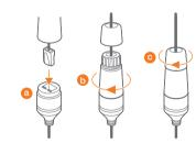
Note: To ensure moisture seal, make sure the o-ring is in place between (a) and (b). In extreme environments use of an outdoor rated sealer
