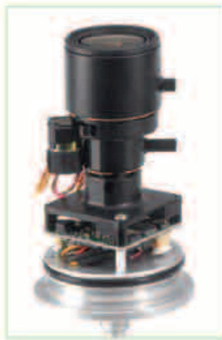
COVER REMOVED SHOWING 2.8-10MM AUTO-IRIS VARIFOCAL LENS
