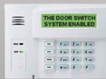
Example of Basic Monitoring Keypad Console
