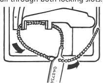
2. Insert and push the bail tip through the tapered end of locking barrel.
