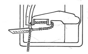
3. Pull bail all the way through until it fits tightly around the locking slots.
