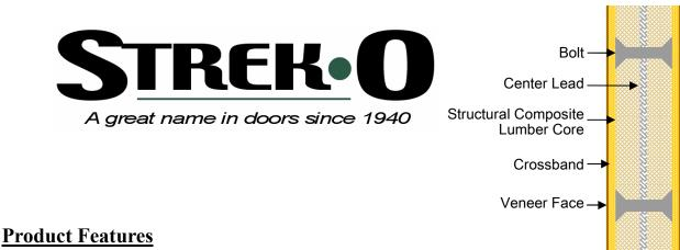
**Construction:** Fully bonded and bolted core on lead over 3/8" lead
