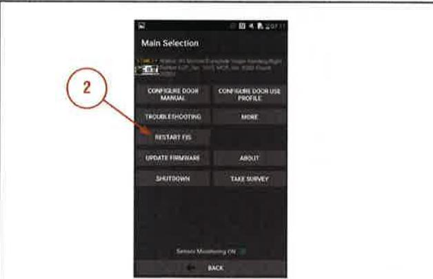
**Step 2:** Press **RESTART FIS** on the **Main Selection** menu. (**FIS** = First Install Sequence).
