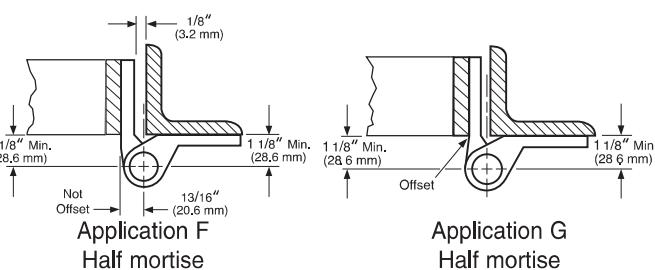
For all full mortise applications the center of barrel should be set 1 1/8" (28.6 mm) from door and frame so welded joints will clear. Leaves can be swaged apart any distance between 1/8" (3.2 mm) to 7/8" (22.2 mm)
