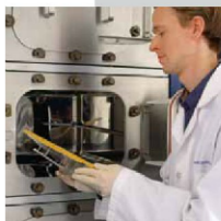
Air Quality Sciences chamber testing verifies that Special-Lite products meet GREENGUARD Certification criteria.
