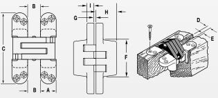
All SOSS Hercules Hinges are shipped with the proper size wood and machine screws unless ordered without. Do not exceed "E" dimension.
