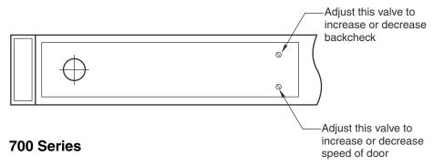
To decrease speed turn valve clockwise. To increase speed turn valve counter clockwise.
