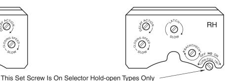
Closing speeds can be adjusted to suit local conditions and requirements. Label on closer face designates the purpose of each adjustment screw. Adjustments are for speed control.
