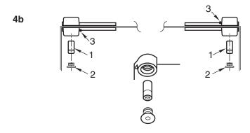
CAUTION: Closer is shipped with Closing Speed valve down, DO NOT FORCE VALVE DOWN.
