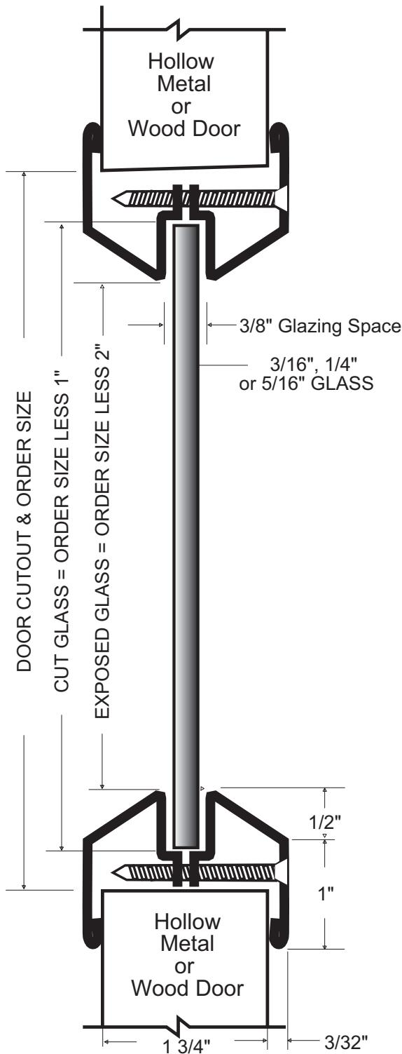
Designed for use on 1-3/4" thick doors manufactured within door industry tolerance of +/- 1/16".
