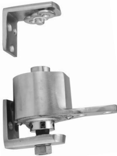
pintle has an adjustment in the bottom attachment with a locking device which permits aligning the gate or setting the gate in desired position. Spring is large enough for heavy duty conditions but the adjustable tension makes it equally suited for light gates.
