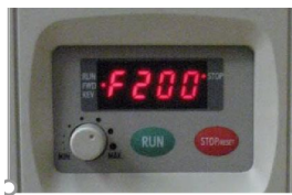
Display of Frequency of Desktop Spindle VFD. Use knob to change Frequency.
