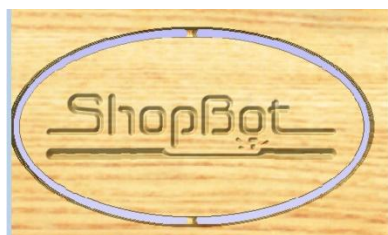
Indication of tabs in 3D simulation, 2D wireframe and 3D toolpath.
