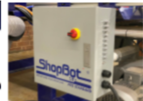
Control Box post May 2020 Separate remote pendant like Desktop Spindle Lockout, soft stop and E-stop on pendant
