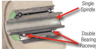
Bearing is insert-molded into the polypropylene hub. This bearing is a single spindle design that cannot become misaligned with use. It is also sealed on both sides after being pre-lubricated with high quality grease.
