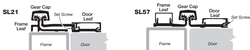
Fig. 2 Door Open Position - Leaf Covers Removed
