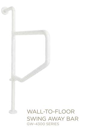
This wall-to-floor mounted swing bar is engineered to move 90 degrees out and back for support when entering or exiting the bath area, swinging outward when in use and tucking back securely against the wall. The swing-away bar is 39" X 3" with a 21" swing arm and locking rotating flange.
