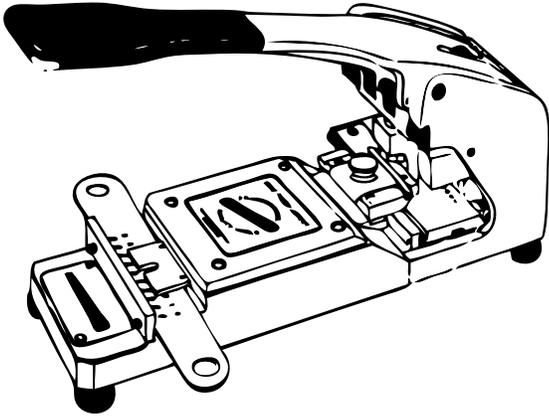
To cut Schlage keys on a rotary cutter code machine, it may be necessary to modify or replace the vise jaw for reliable gripping. Contact your key machine manufacturer directly.
