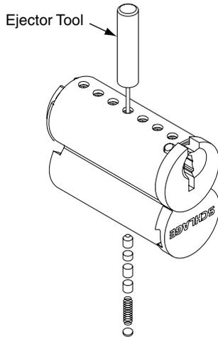
If the problem persists, take your next best guess of where the error is a repeat with another chamber. When all keys operate, you know that the remaining chambers are combined correctly. Recombine the empty chambers. This technique is also used when it is necessary to decombine the core for rekeying.
