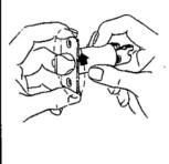
"To adjust: Hold latch with Crank Pin on top as shown in illustration above and rotate the face plate to suit swing of door. This reversible latch unit has a self-adjusting face plate which permits it to be installed on either flat or bevel
