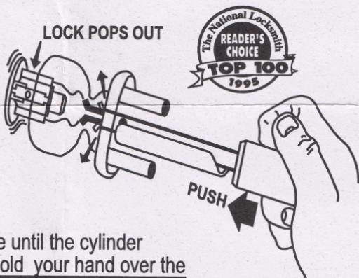
Push in on the tool's red handle until the cylinder pops out of the knob. Do not hold your hand over the face of the lock when trying to remove it from the knob.
