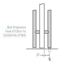
Locking pulls are available for 13/8" to 21/2" thick aluminum, wood or hollow metal doors.
