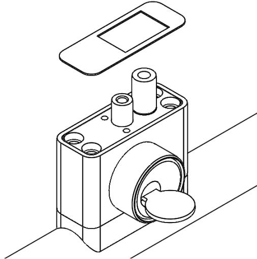
**10** Replace mating pull and device on door and test final function of cylinder by again turning key CCW. This should retract the latch on the Panic Device.
