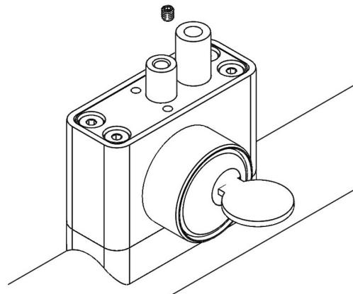
**9** Peel and place new black gasket over top of cylinder housing as positioned prior to removal.
