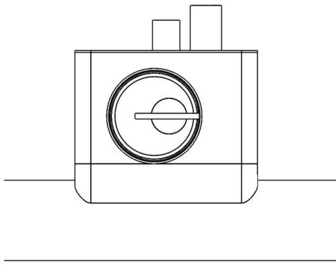
**8** Apply thread locker to 8-32 set screw and replace into cylinder housing to lock cylinder orientation into place.
