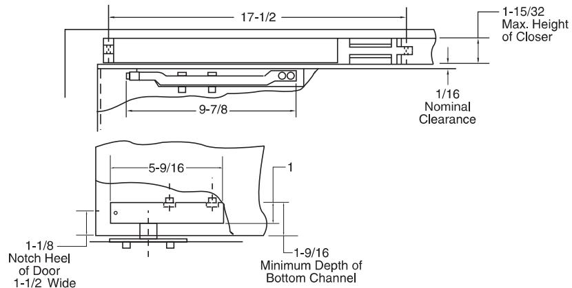
\*Note that mounting channels must be welded into frames prior to shipment to job site.
