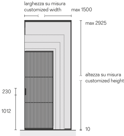
Dimensioni pannelli scorrevoli Sliding panel dimensions
