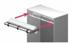
Pull the system forward toward the cabinet front and slide the brackets onto the wooden dowels.
