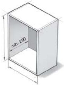
Fig. 3 An internal cabinet depth of at least 290 mm is required for installation.
