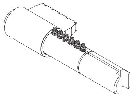
**13** Depress Springs with Knife Tip Sliding Cylinder Shell to Hold Springs in Place
