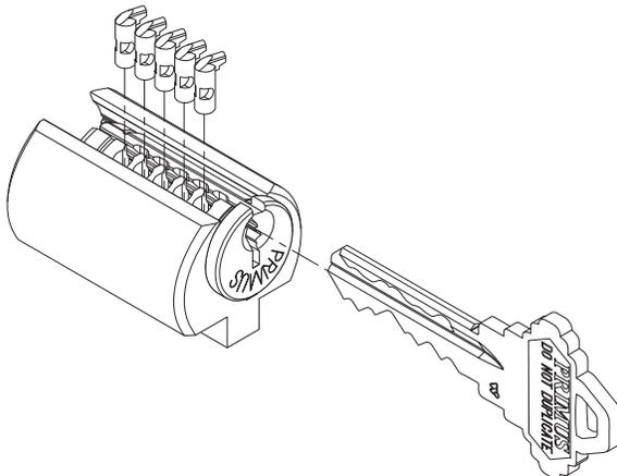
**11 Load Top Pins and Springs into Loading Tool**
