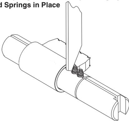
**14** Rotate Cylinder Shell to Align Chambers
