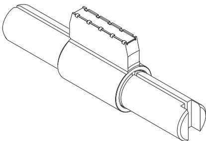
**15** Insert Knife Into Groove in Loading Rod
