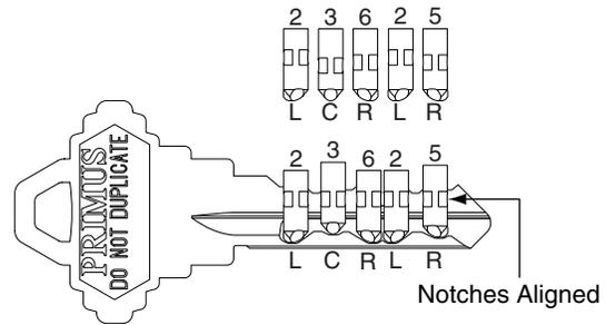
Each of the side cuts raise and swivel the finger pin in order to align the notch in the pin to the notch in the side bar.
