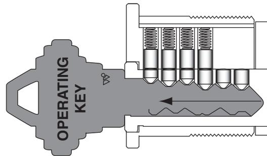
The operating key cannot be removed in the lockout position because the back two pins are unable to disengage from the key.
