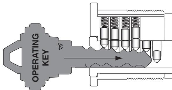
The operating key cannot enter the cylinder because the back two pins are not able to settle into their biting spaces on the key.
