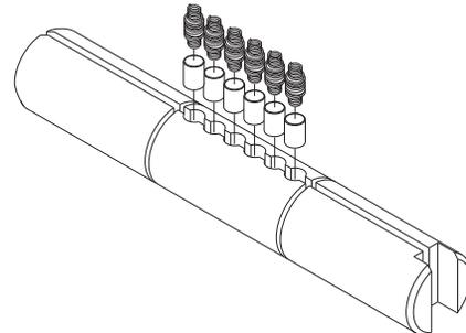
**12 Place Rotated Cylinder Shell on Loading Rod**
