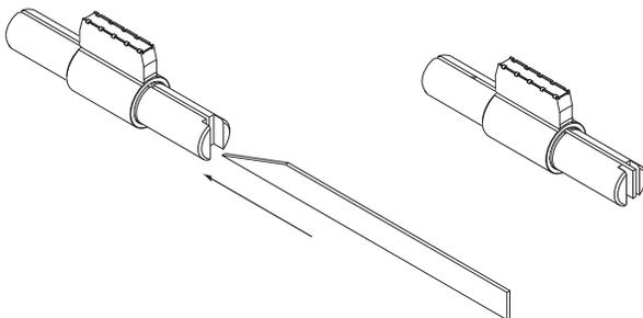
**16** Remove Plug From Holder and Rotate 45°
