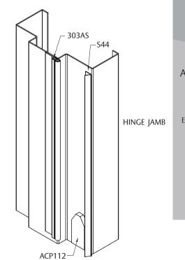
System Detail of an Acoustical Seal Set for Door & Frame
