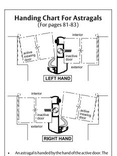
hand of the active door is determined by the position of the hinges on the door, when viewed from the outside (the key side).
