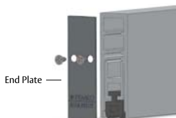
Figure 4 - Properly Installed End Plate
