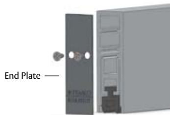
Figure 4 - Properly Installed End Plate
