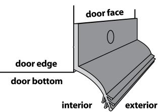
At the door bottom (for both one piece and sectional), install on exterior (outside) door face.
