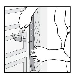
At the top and sides (for sectional doors), install on the jambs.
