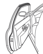
Closed Cell Sponge Neoprene Tape installed as car door weatherstrip.
