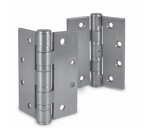
BB1068 & BB1099 series hinges are full mortise heavy-duty hinges. Made from the highest quality materials. These hinges are suitable for high traffic industrial door applications and are recognized for value while delivering lasting performance.
