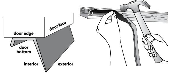
The long flap should face the exterior (outside) of the garage.
