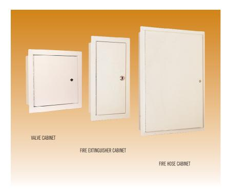
**Detention Series Cabinets** provide the specifier with the substantial unitized design of 12 gauge cold-rolled steel construction for maximum security facilities. All corners are mitered and ground smooth to eliminate any dangerous projections. The heavy-duty continuous hinge adds to the secure features of these cabinets.
