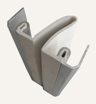
Nystrom's Seismic Elastomeric Ceiling System uses an aluminum channel attached to the grid system above the sight line. The finished Santoprene seal comes in four colors to match your surrounding substrate and finish material. This system accommodates seismic movement.
