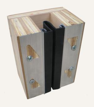
This Seismic Elastomeric Drywall System limits the sight line of the expansion joint by using a drywall bead to mount the system outside the joint opening with a finished tape and mud process. The finished Santoprene seal comes in four colors to match your surrounding substrate and finish material. This system accommodates seismic movement.
