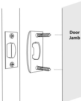
Attach the strike plate to the door jamb using 3/4" long wood screws.
