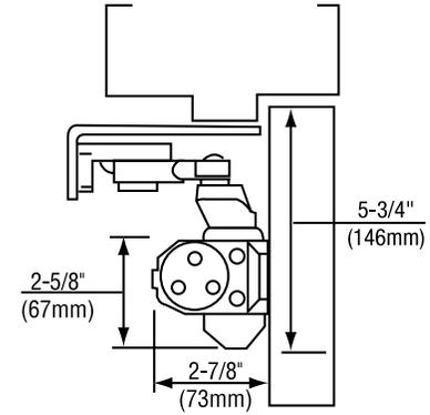
Mounting holes for closer body are spaced 3/4" (19mm) vertically x 9-1/16" (230mm) horizontally.
