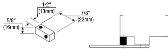
**Standard - #2019S Spacer Block:** For use where a narrow frame soffit does not provide adequate support for the soffit plate. Supplied as standard with all parallel rigid arm closers. For use on frame with either 1/2" (13mm) or 5/8" (16mm) high frame stop.
