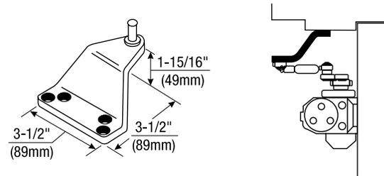
**Extra-Clearance - #2018S Offset Soffit Plate:** For use where the need for additional clearance prevents use of the standard soffit plate. This plate mounts to the frame soffit to provide up to 2" (51mm) of clearance when a separate overhead door holder is used. Standard mounting requires a 2-5/8" (67mm) wide frame soffit. It may also be used where unusually high frame stops or weatherstripping prevents the use of other soffit plates.
