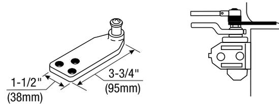
**Molded/Bull Nose Trim - #2403-3/4 Bracket:** This bracket is similar to-but longer than-the 2403B bracket. It is designed to accommodate frame rabbets from 2" to 2-7/8" (51 to 73mm) deep.
