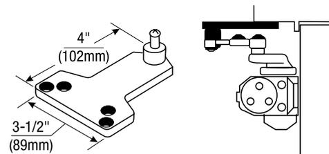
**Blade/Applied Stop - #2018D Soffit Plate:** For use where a blade or applied stop does not permit installation of the standard soffit plate. Mounts to either the frame soffit or rabbet. Since this soffit plate projects 7/8" (22mm) less than a standard soffit plate, it requires a minimum frame reveal of 1-1/2" (38mm). Permits closer to clear up to a 5/8" (16mm) high frame stop.
