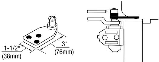
**Molded/Bull Nose Trim - #2403B Bracket:** For use where the door frame has molded or bull nose trim which will not accept a standard non-hold open shoe. The bracket is mortised into the frame rabbet, and projects beyond the face of the frame. It will accommodate a frame rabbet up to 2" (51mm) deep.
