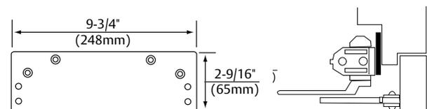
**Low Ceiling Clearance - Overhead Door Holder - #1687 Drop Plate:** For use where the ceiling clearance is between 1-3/4" and 2-5/8" (44 and 67mm). Or for use where an overhead door holder prevents normal top jamb mounting. This places the centerline of the arm mounting screws at 2-1/8" (54mm) from the top of door.
