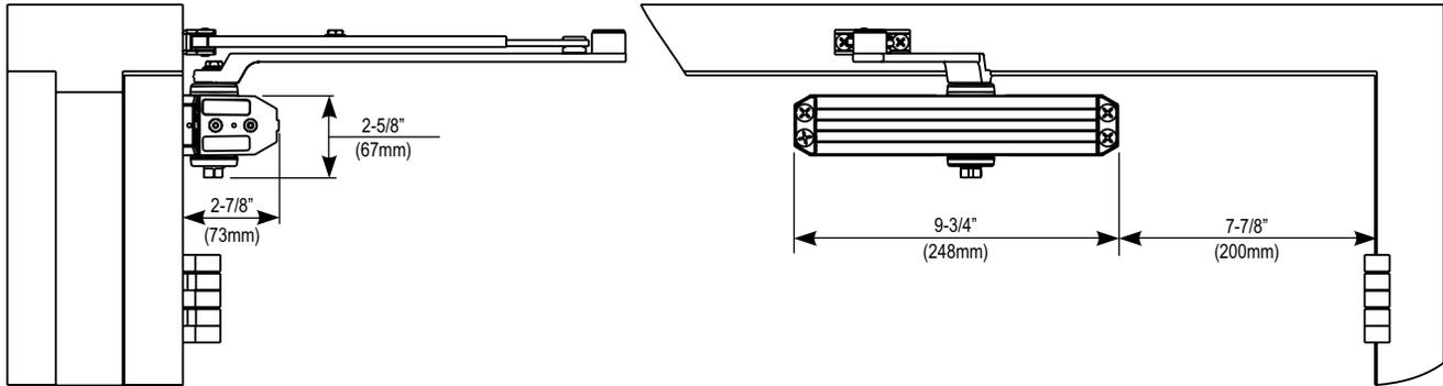
Mounting holes for closer body are spaced 3/4" (19mm) vertically x 9-1/16" (230mm) horizontally.
