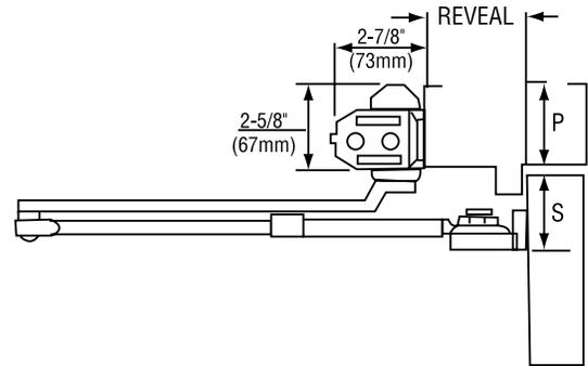
Mounting holes for closer body are spaced 3/4" (19mm) vertically x 9-1/16" (230mm) horizontally.
