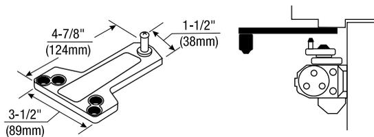
**Standard Installation - #1618A Soffit Plate:** This soffit plate is supplied standard with parallel arm closers. It can be mounted where the frame soffit is as narrow as 1" (25 mm).
