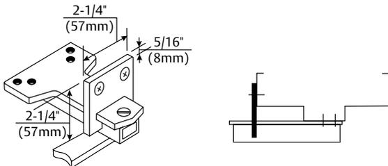
**Additional Support - #6190 Reinforcing Bracket:** Standard for use with all parallel arm Unitrol Door Controls. Provides additional support to the soffit plate on installations with door frame reveals from 1-7/8" to 4-5/8" (48 to 117mm).
