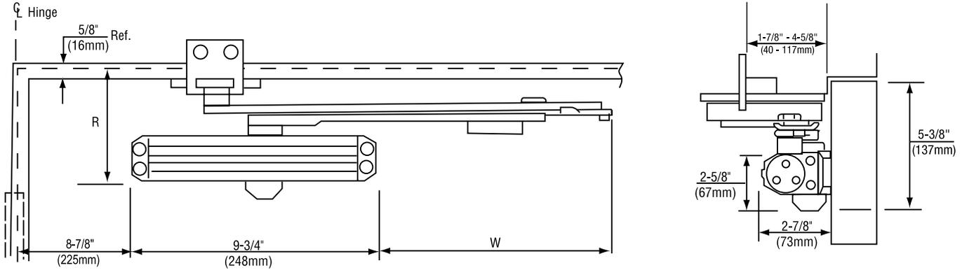
Mounting holes for closer body are spaced 3/4" (19mm) vertically x 9-1/16" (230mm) horizontally.
