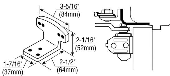
**Molded/Bull Nose Trim - #80 Bracket:** For use where the door frame has molded or bull nose trim which will not accept a standard hold open shoe. It is mortised into the frame rabbet, and projects beyond the face of the frame. It will accommodate a rabbet up to 2" (51mm) deep. This bracket is used in combination with the standard hold open mounting shoe.
