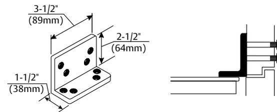
**Flush Rabbeted Transom - #2022 Angle Bracket:** Optional for use with all parallel arm Unitrol Door Controls. For use where rabbeted or flush transom conditions prevent installation of the soffit plate assembly. This bracket fastens to the overhead transom to provide a mounting surface for the soffit plate assembly.
