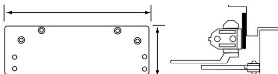
**Overhead Door Holder - #1688 Drop Plate:** For use where a overhead door holder prevents normal top jamb mounting. This places the center line of the arm mounting screws at 3-1/2" (89mm) from the top of the door.
