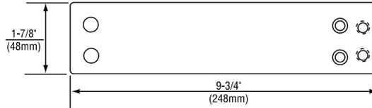
**1699 Adapter Plate:** Converts old 1602/1603 closer installations with  $\frac{3}{4}"$  (19mm) x  $8\frac{3}{16}"$  (208mm) - spacing to new 1603 using existing mounting holes in door or frame.
