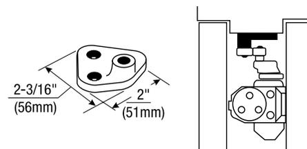
**Mounting Between Doors - #2018 Soffit Bracket:** For use where insufficient space between companion doors does not permit use of other soffit plates. This bracket permits mounting of the closer between doors with as little as 3" (76mm) of header space. Permits closer arm to clear up to 5/8" (16mm) high stop.
