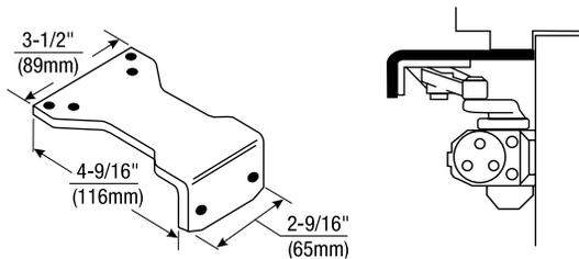
**Parallel Hold Open - #1628H Adapter Plate:** This Adapter Plate is supplied standard with all parallel arm hold open closers. It can also be used to convert regular arm or top jamb hold open arms to parallel arm installation. It can be mounted where the frame soffit is as narrow as 1" (25mm).
