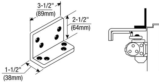
**Flush Transom - #2022 Angle Bracket:** For use where rabbeted or flush transom conditions prevent installation of a soffit plate. Used in combination with the 1618A soffit plate, or may be used in combination with the 2018S soffit plate when it is necessary for the closer arm to clear a separate overhead door holder.
