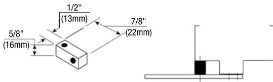
**Standard - #2019S Spacer Block:** For use where a narrow frame soffit does not provide adequate support for the soffit plate. Supplied as standard with all parallel rigid arm closers. For use on frame with either 1/2" (13mm) or 5/8" (16mm) high frame stop.
