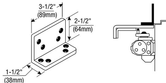
**Flush Transom Hold Open - #2022 Angle Bracket:** For use where rabbeted or flush transom conditions prevent installation of the standard 1628H hold open adapter plate. It is used in combination with the 1628H adapter plate.
