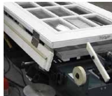
Quick-adjust jamb supports enable convenient hinge application.
