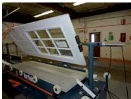
Door Flipping Device eliminates manual lifting & reduces chance for injury.
