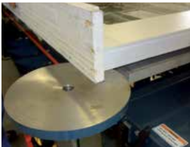
Corner support plates provide a flat surface for squaring jambs and freeing both hands for installation of fasteners.
