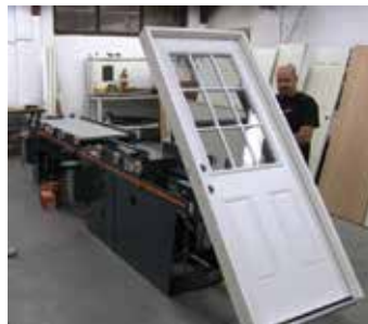
Second stage provides brick-mould application station and tilts finished unit to upright for easy off-loading.
