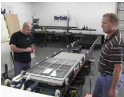
Lite Insertion platform expedites lite kit installation.
