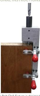
The Extension Flush Bolt Drill Fixture is designed to drill a ½" diameter hole up to 16" long in a door for the extension rod on a flush bolt. The unit is primarily designed to be used on 1-3/4" thick doors and to position the center of the hole ¾" from the door edge. Shims can be used for applications on thinner doors or if the hole location is to be less than ¾" from the edge.
