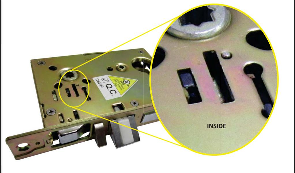
HOW TO REVERSE LOCKING PIECE FROM FLUSHED SIDE TO HOLLOW SIDE: Use a tool, preferably a flathead screw driver that will fit into the locking piece slot (FIGURE 1). Push the locking piece down (FIGURE 2).
