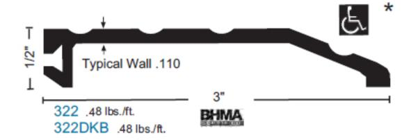
\* when installed with the non-beveled edge FLUSH with flooring, or where no greater than 1/4" vertical rise occurs.
